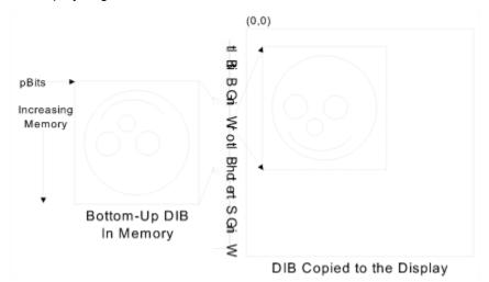
Bottom-Up DIBs are flipped when copied to the display
